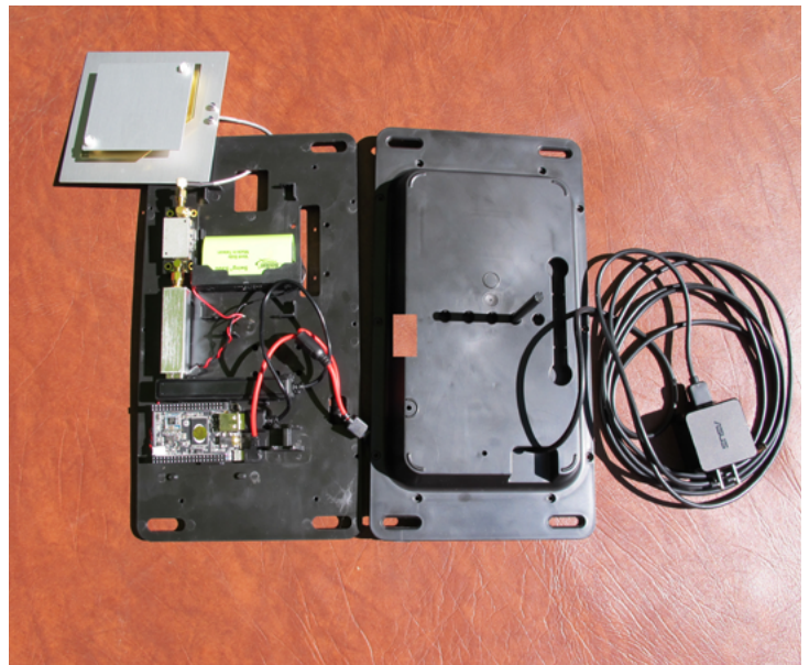
Outernet Lantern disassembled: L-band antenna is at upper left, power cord is at right. (Courtesy: Kenneth Barbi)
