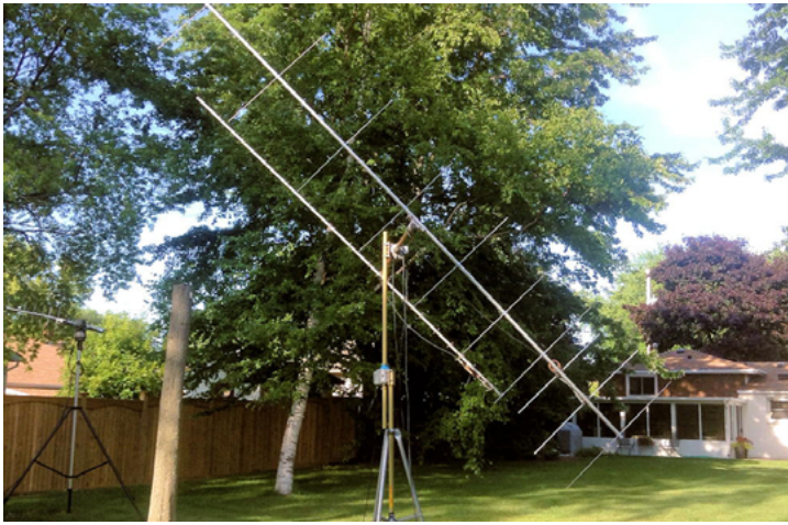
A very effective portable satellite antenna array can be made using a pair of old Alliance (Genie) U-110 television rotators, a set of 2-meter and 70-cm “terrestrial” Yagi antennas along with a 3 or 5-foot rooftop television antenna mast. (Courtesy: Author)
