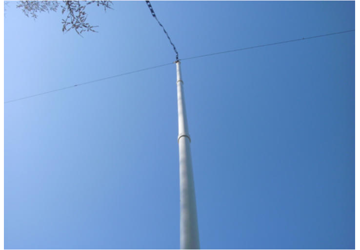
Center of my old 102-foot dipole, 35 feet up. At 500 kHz, it would need to be nearly 1000 feet long and 1000 feet up above ground; at 468 MHz, it would be a foot long. (AC0LW photo)
