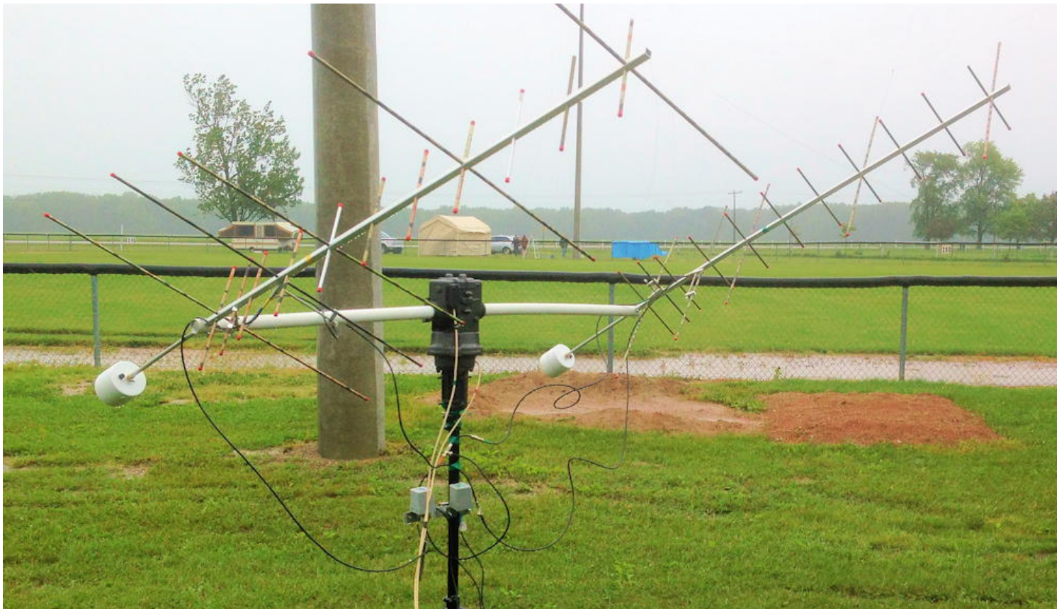
ARRL's Field Day is a great opportunity to try out different portable satellite antenna designs. Here, a pair of Arrow-style antennas are used with 75-Ohm phasing lines to achieve a "circular-like" radiation pattern. The rotator is a Yaesu G-5400 AZ/EL combo and the tripod is a DJ speaker stand, both obtained from eBay. (Courtesy: Author)
