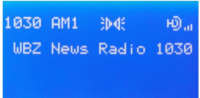
(Above) WBZ-AM, Boston, as received a few years ago in central Virginia, using a Radio Shack tunable AM loop antenna on a Sangean HDT-IX receiver. At a distance of more than 480 miles the HD-Radio digital signal locked in, at least for a while, offering FM-quality audio while it lasted. Unfortunately, WBZ does not carry Red Sox baseball today. (KS4ZR photo)
