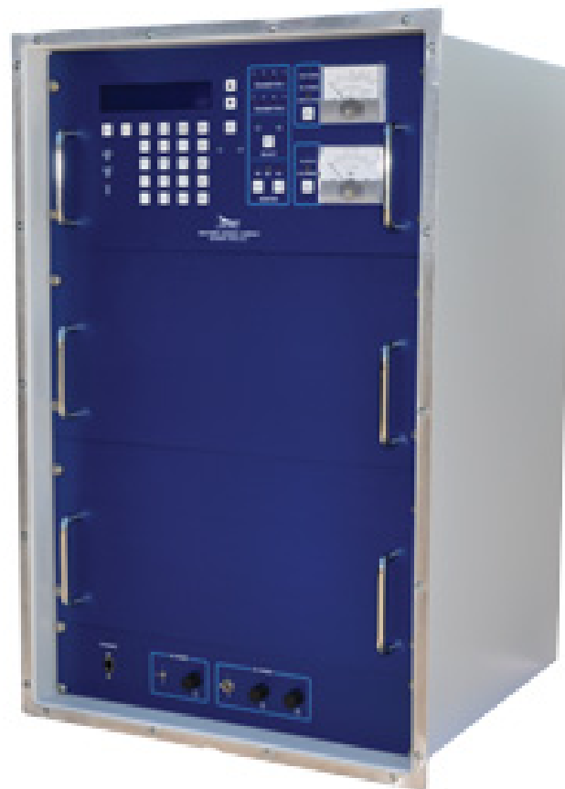
Southern Avionics manufactures NDB transmitters that can be configured to transmit from 10 to 1,000 watts. The SE Series NDB transmitter (pictured above) uses state of the art technology including powerful Renesas© Microcontrollers and Analog Devices© Direct Digital Synthesizers to provide accurate beacon signals in power ranging from 10 Watts to full rated carrier power. SE Series transmitters feature: 125-Watt carrier power; Programmable for any frequency from 190-650 kHz; Optionally Programmable from 650 to 1250 kHz and 1500 to 1800 kHz.. (Photo and caption courtesy of Southern Avionics)
