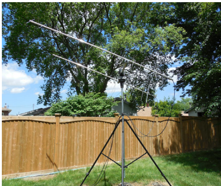
A portable satellite antenna array can also be used in a semi-permanent (or even permanent!) setup. My principle satellite antennas consist of an M2 Model 2MCP14 for 2-meter and a M2 436CP30 for 70-cm. The array is mounted on a metal cross-boom with a Yaesu G-5400 rotator and an MFJ Model 1921 Heavy Duty tripod. Mounting the 2-meter antenna at a 45 degree angle on the cross-boom helps to minimize interference to the circularly polarized pattern. (Courtesy: Author)
