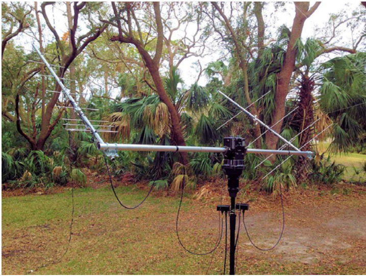
During the first few months of 2017, I very successfully used an M2 Antenna Systems “LEO Pack” and an old Yaesu G-5400 Az/El Rotator combo at our family’s rental home on Fripp Island, South Carolina. (Courtesy: Author)
