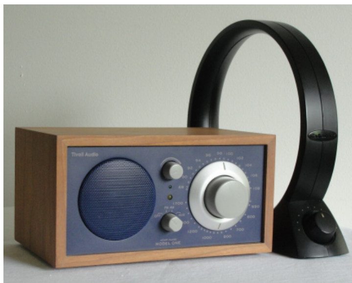
The Radio Shack AM loop antenna in action with a Tivoli Audio Kloss Model One AM/FM radio. (KSRZR photo)
