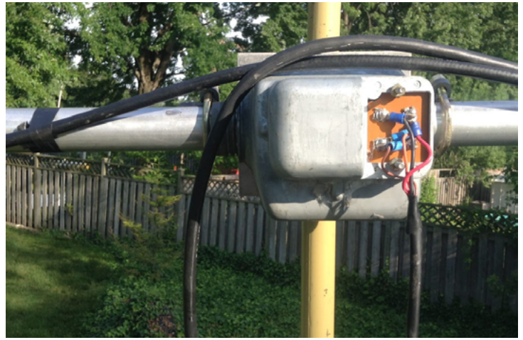
The old Alliance (Genie) U-110 television rotators featured a “through the rotator” design that works well for the elevation side of an Az/El satellite rotator arrangement. However, you may have to fashion your own cross boom rotator plate. (Courtesy: Author)
