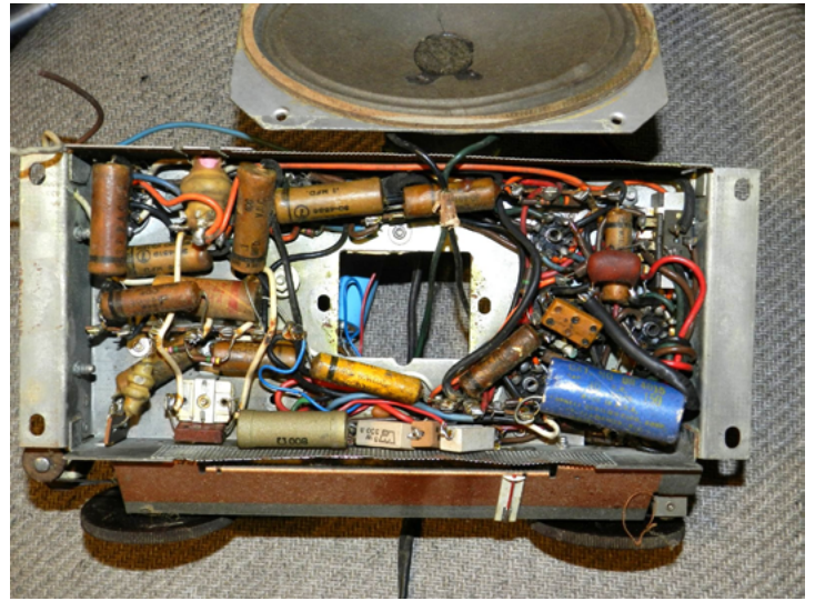
Philco 46-350 chassis with original wax capacitors. (KB8TAD photo)
