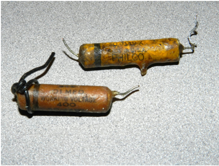
Cap with wax stalactite and cap with one turn 'gimmick' choke. (KB8TAD photo)
