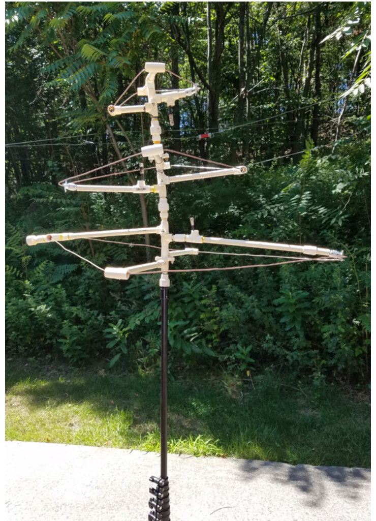
My new version of my VHF and above loop antennas now includes a 222 MHz antenna. (N6CL photo)
