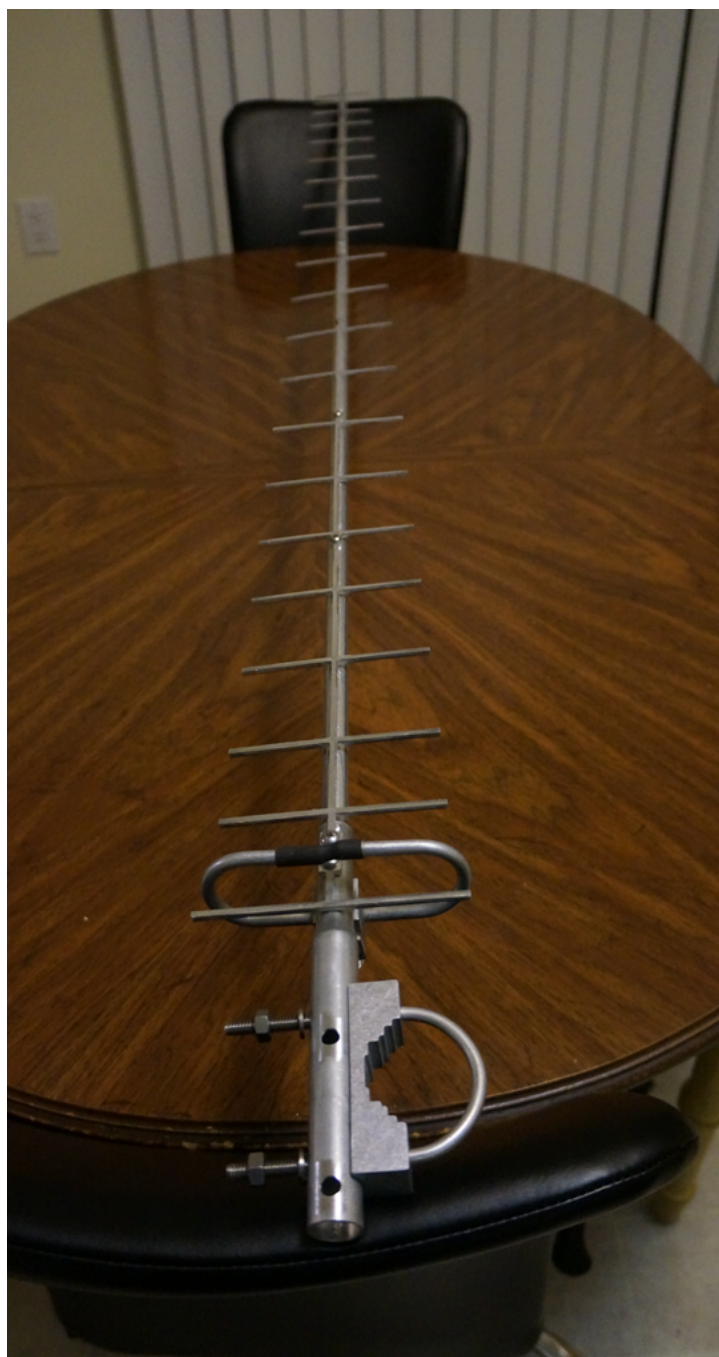
My new M2 23CM22EZA 1296 MHz rover antenna spread out across my dining table just after I assembled it. (N6CL photo)
