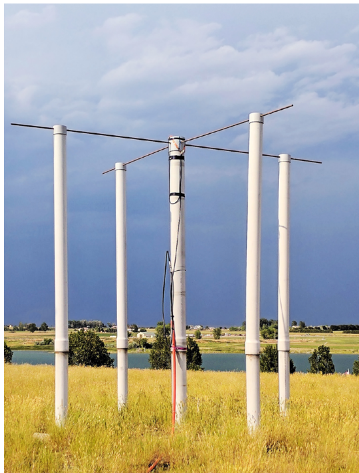
Experimental antenna for 25-MHz WWV. (Courtesy NIST)
