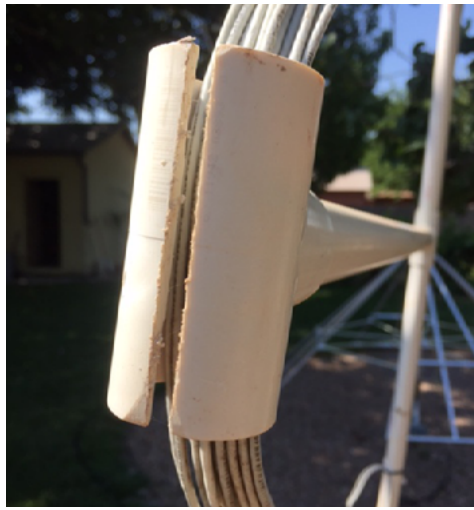
The author's 4-foot VLF loop (left) and close-up of cross-arm that holds the wires. (Courtesy of the author)
