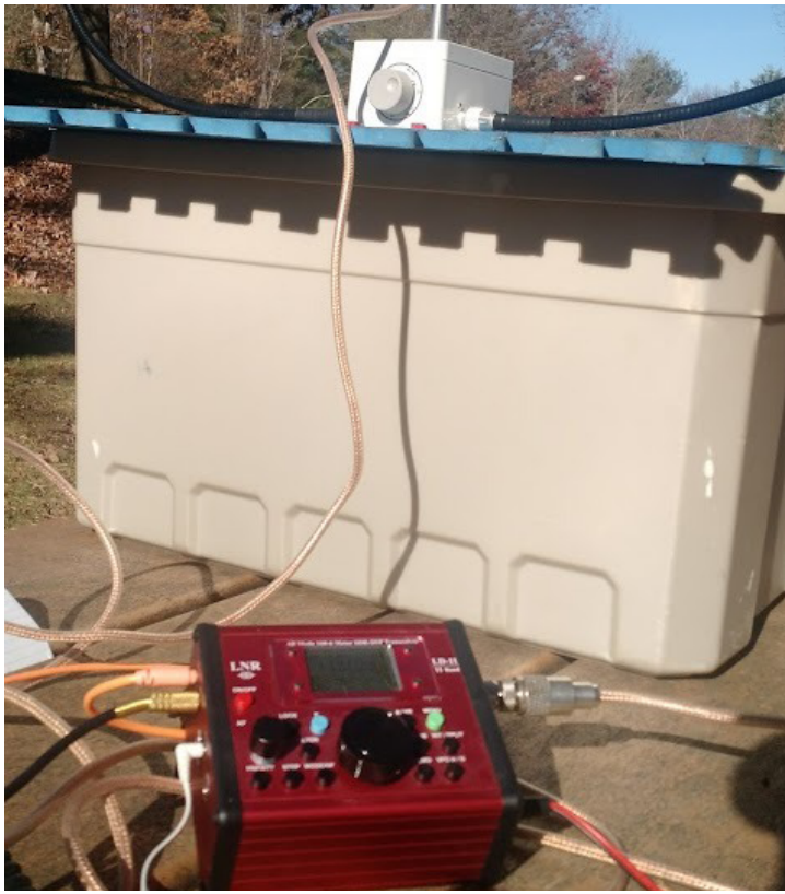
LnR Precision's LD-11 (see October 2016 TSM for review) pairs beautifully with the W4OP loop. The lack of an internal LD-11 ATU is no problem since all of the tuning/matching is accomplished on the loop. (Photo by Thomas Witherspoon K4SWL)
