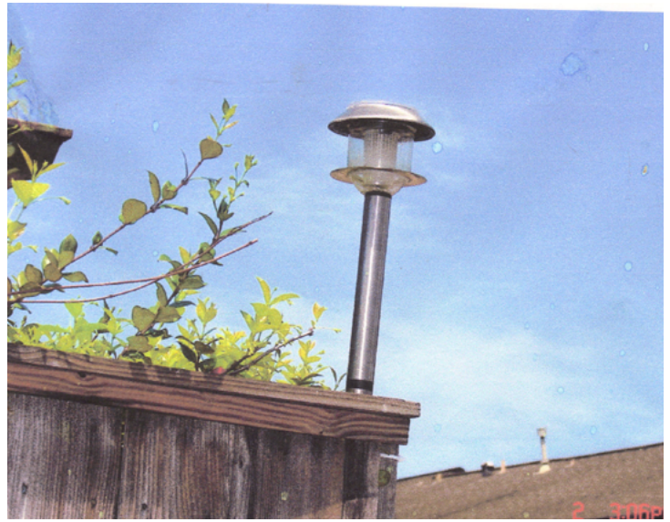
One of my readers sent me this shot of his stealthy DX500 active antenna, on the back fence with an LED solar-powered lamp on top. (From author's photo archive)
