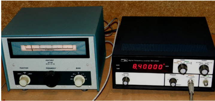
HG-10B on the 6-meter range. The 8.400 MHz multiplied by six is intended for a transmitter for 50.4 MHz. (KB8TAD photo)
