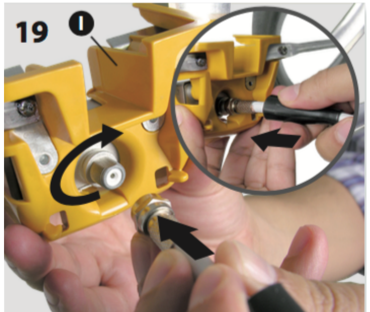
Part of Televes DAT-790 instruction sheet, shows connecting 75 ohm coax to the antenna's driven elements. (Courtesy: Televes)
