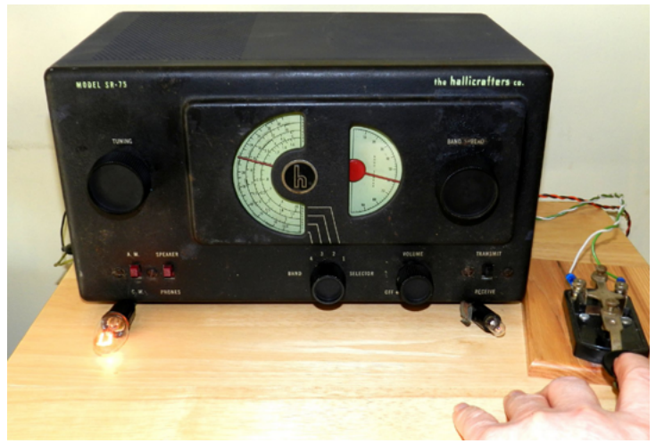
Completed SR-75 lighting both a dummy load bulb and a #1804 tuning bulb (near the key, rated at 60 mA at 4 volts which I substituted for a #49 (60 mA at 2 volts). (KB8TAD photo)
