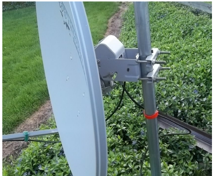
Horizon-to-horizon motor for 36-inch Ku-band dish. (Courtesy: Mario Filippi N2HUN)
