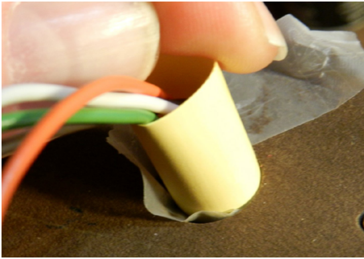
Fitting the heat shrink into the recessed jack location. KB8TAD photo)
