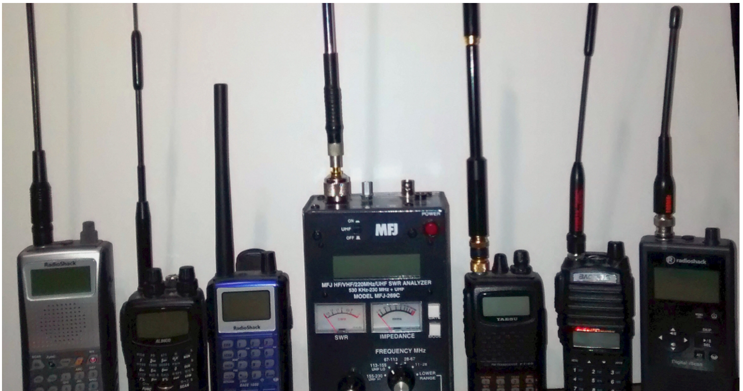
The author's array of amateur radio HTs and portable scanner receivers sporting a variety of antennas. His MFJ-269C antenna analyzer is in the center. (Courtesy of the author)
