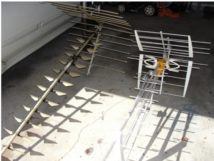
Televes VHF/UHF-TV antenna compared to old Channel Master UHF-only TV antenna—basically, the same number of UHF elements on a much shorter boom with the addition of VHF elements at the back. (KS4ZR photo)
