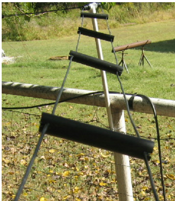
A good view of some homemade ladder line. (Photo by author)
