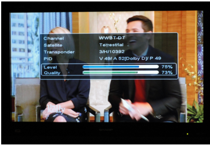
VHF-TV WWBT channel 12 (with just 26 kW ERP) from 45 miles away using the Televes amplified antenna. And, the antenna isn't properly pointed yet. (KS4ZR photo)
