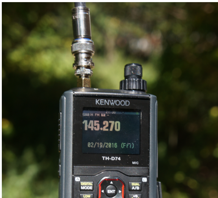
How the compression male BNC connector is connected to the female BNC to male SMA adapter that is installed onto the hand-held radio. (N6CL photo)
