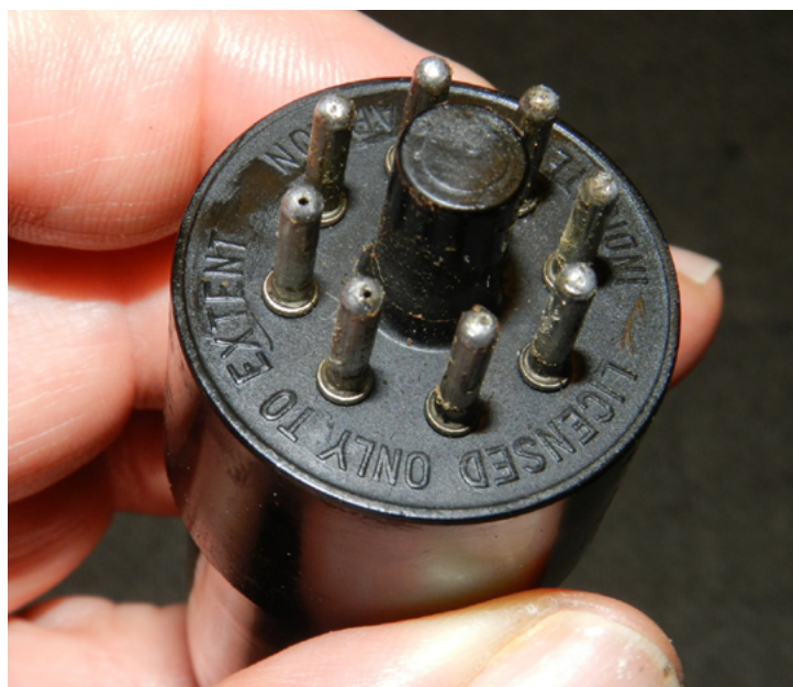
Bottom of intermittent 6SA7. Can you spot the problem? (KB8TAD)
