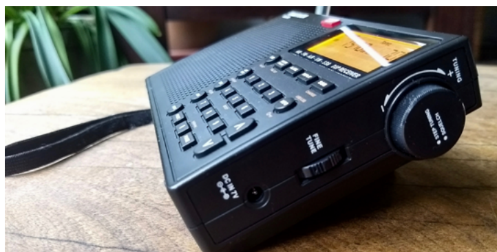
Both the main tuning encoder and the Fine Tune control are on the right side of the AR1780. (K4SWL photo)
