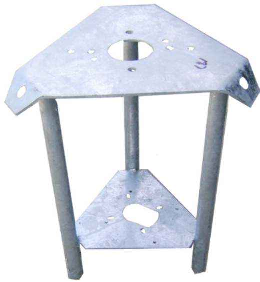
Rohn 25G rotator and thrust bearing shelf fits atop a Rohn 25G tower section. The rotator is bolted to the bottom shelf with the 2 or 3-inch mast going through the thrust bearing on the top shelf. (Courtesy: Amazon)
