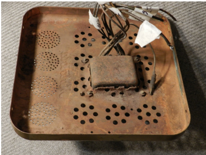
Rusty cover with hole cut for power transformer. (KB8TAD photo)
