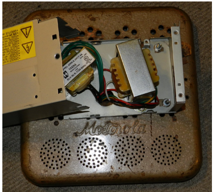
Bottom cover with new transformers bolted inside case from a defunct computer power supply. (KB8TAD photo)
