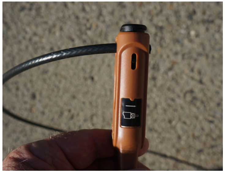
How to insert the coaxial cable into the trigger strip tool. (N6CL photo)
