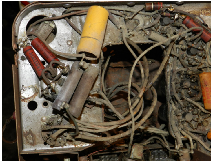
Chassis bottom of converted car radio as found. (KB8TAD photo)
