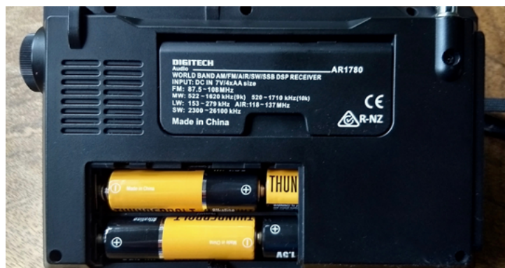
Very pleased the AR1780 uses standard AA cells. Note that the frequency coverage silk screened on the back stand is incorrect. (K4SWL photo)
