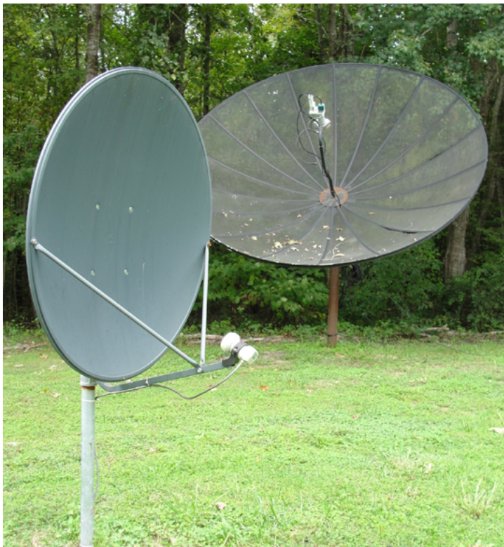
90-cm (about 36-inches) Ku-band dish in foreground with 10-foot C/Ku-band dish in background. The small dish is fixed on Hispasat at 30 degrees west. Positioned over the Atlantic Ocean, it serves both eastern and western hemispheres. This was the satellite to go to for Cuban hurricane coverage. (KS4ZR photo)
