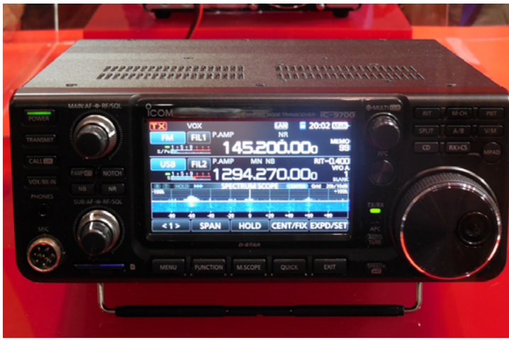
One of the new radios featured at the show was the ICOM IC-9700, a VHF/UHF, all-mode, and satellite-capable radio. It features variable power output of 50W for VHF and UHF and 10W output on 1.2 GHz. Despite my questions, no word was given on price or North American availability. (Courtesy: Author)
