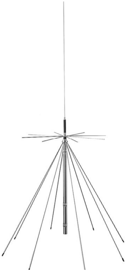
Diamond D3000N discone antenna ($135) is 67 inches high and receives from 25 to 3000 MHz and can also be used for transmit on 50, 144, 430, 900 and 1200 MHz ham bands (under 100 watts on 144 up, and 20 watts on 6 meters). (Courtesy: Universal Radio)
