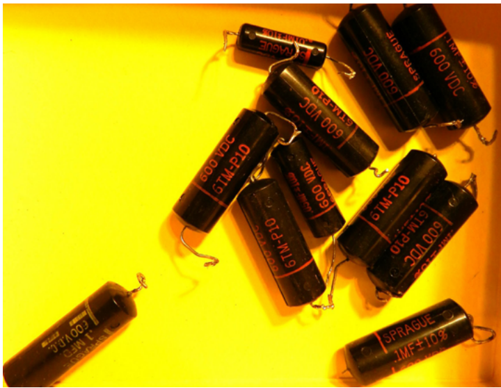
Capacitor surprise, Sprague 6TM capacitors that were not leaky. The one capacitor on the lower left is not a 6TM and was the only leaky cap. (KB8TAD photo)
