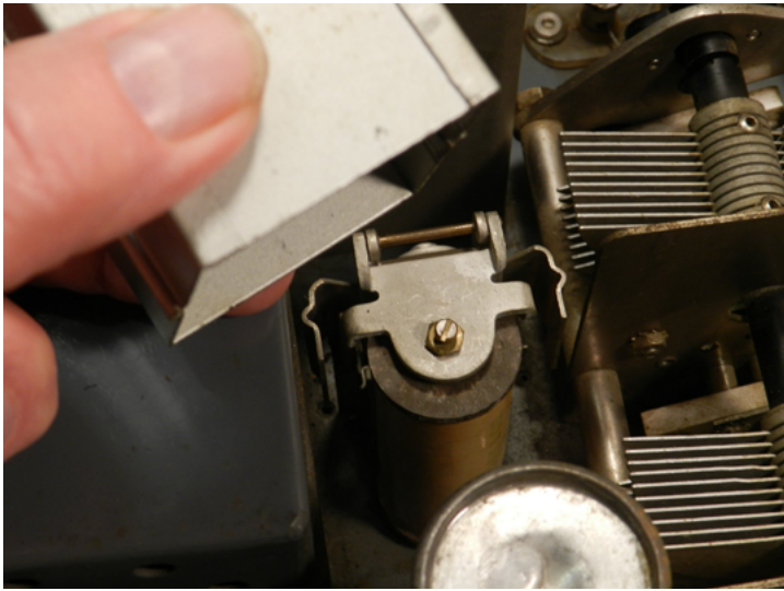
CONS relay with cover removed. (KB8TAD photo)
