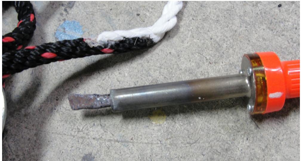
Left: Block and tackle from Tractor Supply ($50) turns an antenna-raising project into a one-man ordeal. (Courtesy: Tractor Supply) Right: 40-watt soldering iron with modified tip for splicing synthetic rope. The type of rope used with the block and tackle was braided and the spliced rope was twisted, but they both appeared to be Polyester. I overlapped the two by about two inches, melted and smoothed the connecting edges so that they would pass through the block and tackle pulley sets. (KS4ZR photo)
