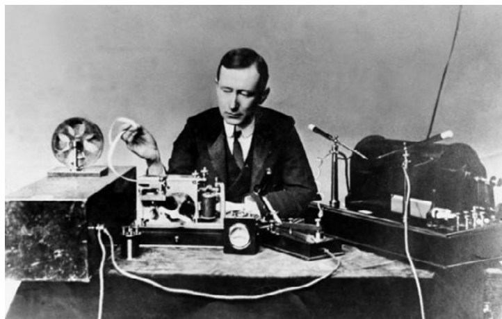
Electrical engineer/inventor Guglielmo Marconi with the spark-gap transmitter (right) and coherer receiver (left) he used in some of his first long distance radiotelegraphy transmissions during the 1890s. (By Published on LIFE [Public domain or Public domain], via Wikimedia Commons)
