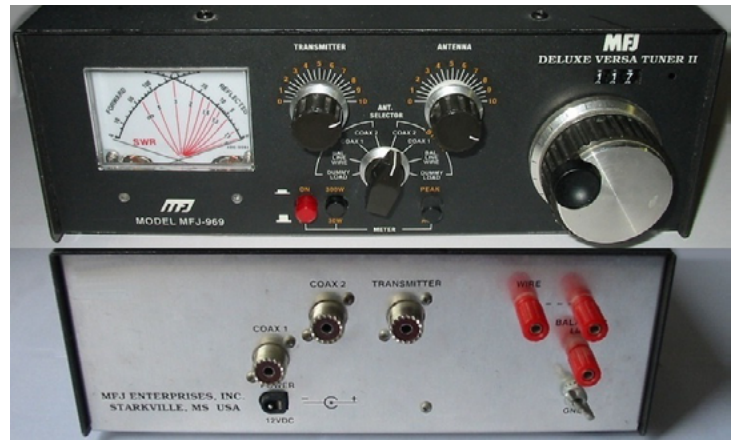
Front and back views of MFJ's excellent Model 969 tuner. (Courtesy MFJ Enterprises)
