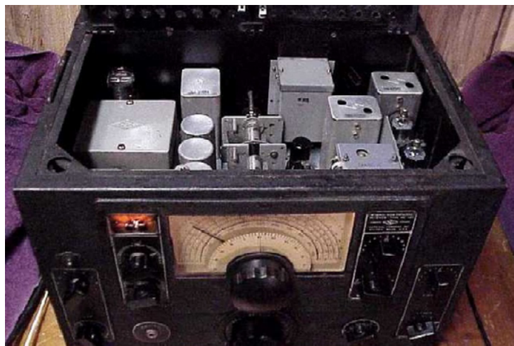
National NC-120 moving coil radio, made for the Navy as the RAO-2. (KB8TAD photo)
