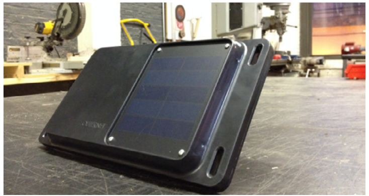
Latest version of Outernet’s Lantern L-band data receiver, a self-contained receiver, antenna, amplifier and data processor. (Courtesy: Outernet)
