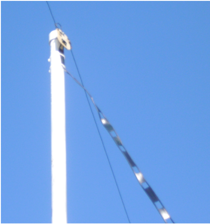
One of the author's big dipoles, fed with ladder line. (Author's photo)
