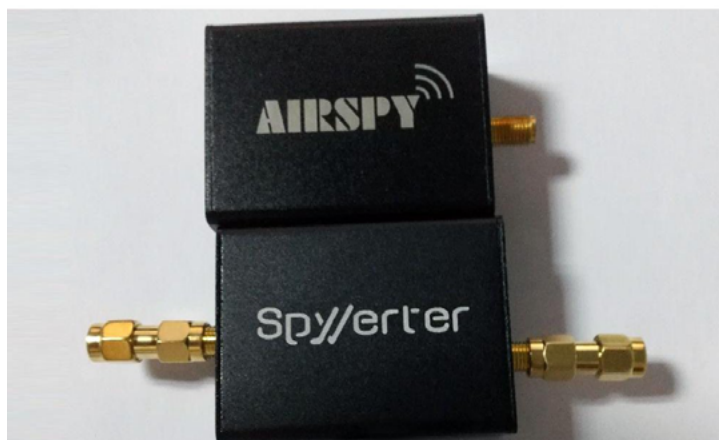
Wide coverage SDRs such as the Airspy R2 and Spyverter (above $218) includes the accessories of each item for coverage from 1 kHz to 1800 MHz. (Courtesy: AirspyUS)
