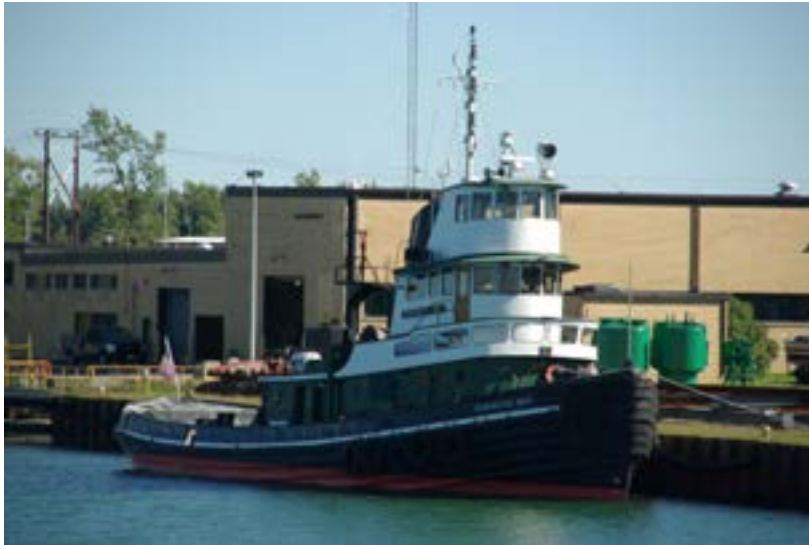
US Seaway tug Robinson Bay which is used to remove and deactivate aids to navigation for the winter
