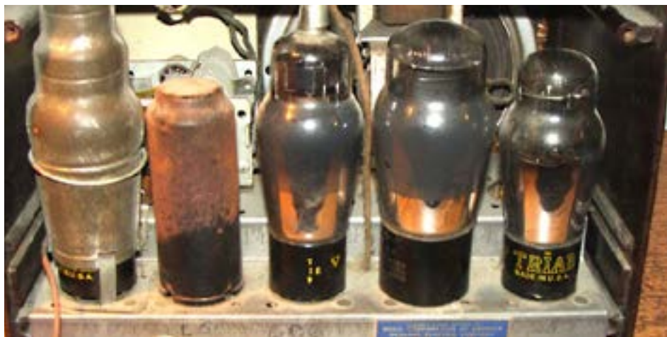
The back of this flea market AC/DC set is missing, dangerously exposing the chassis and other metal parts, which could be hot to ground. See text for suggestions on replacing the deteriorated line cord.
