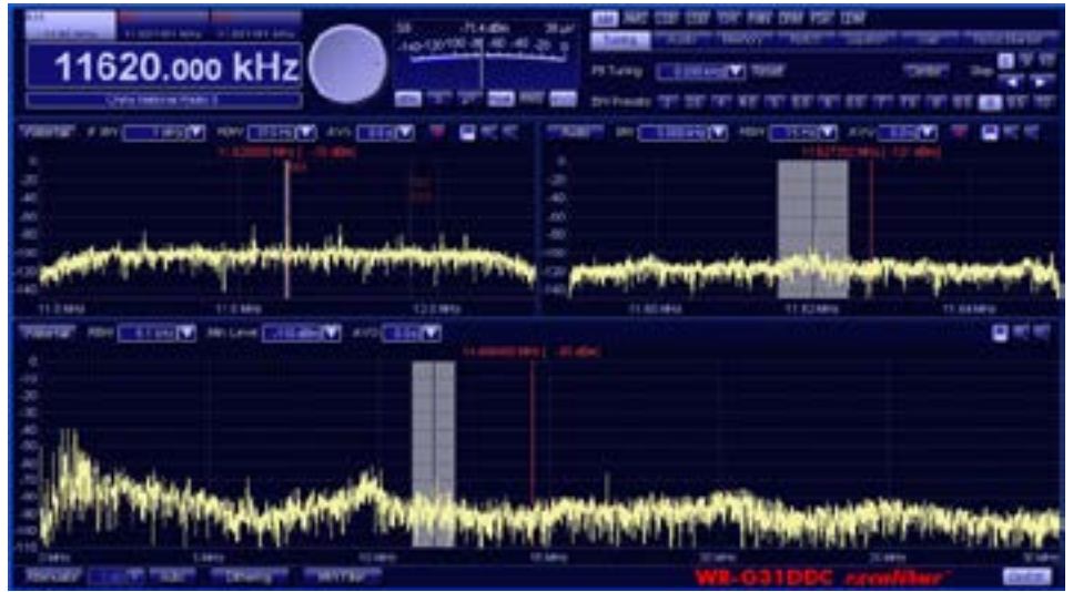
Here’s the display side of the WiNRADiO G31DDC Excalibur Software Defined Radio. With a frequency range of 9 kHz to 49.995 MHz with 1 GHz/s search speed, 50 MHz wide real-time spectrum display and built-in audio recorder with a USB 2.0 interface, this is state-of-the-art radio today. (Courtesy: WiNRADiO)
