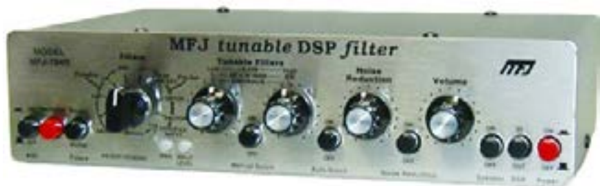
Modern shortwave radios and amateur transceivers have built-in Digital Signal Processing. But, many shortwave listeners and hams have older rigs not so well equipped. MFJ's 784B Tunable DSP filter can be just the thing to help block out adjacent channel interference and dull the effects of QRN and local QRM. At $250 from Universal Radio, it's not cheap, but then, neither is buying a new rig! (Courtesy: MFJ Enterprises)
