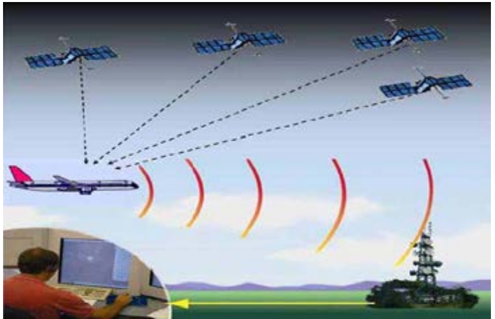
How ADS-B Works: The aircraft determines its position through GPS; that position is downlinked to a ground station to be added to other data and rebroadcast to all ADS-B equipped aircraft. (Copyright Air Services Australia, used by permission)
