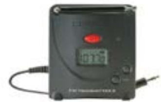
AOR's LA800 amplified loop antenna (left) works from 10 kHz through 500 MHz and measures two feet eight inches across. Control box (right) output is via a BNC jack. A 3.3 foot BNC to BNC patch cable and 33 feet of low loss coax cable is provided. This antenna operates from 12 VDC or via the supplied AC wall adapter.
