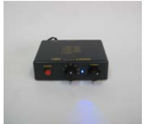
AOR's LA800 amplified loop antenna (left) works from 10 kHz through 500 MHz and measures two feet eight inches across. Control box (right) output is via a BNC jack. A 3.3 foot BNC to BNC patch cable and 33 feet of low loss coax cable is provided. This antenna operates from 12 VDC or via the supplied AC wall adapter.
