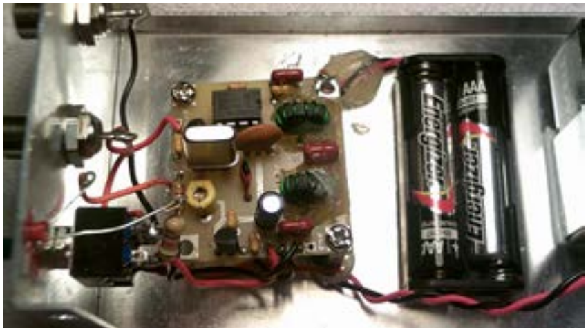
This longwave converter costs just $14 and provides respectable performance for DXing. (Photo courtesy of Ron Smith)
