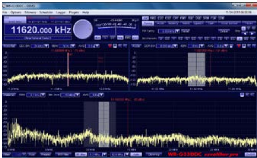
Spectrum display from WiNRADiO WR-G33DDC Excalibur Pro, an excellent example of digital radio technology. Note that the bottom screen shows the entire HF spectrum from 0 to 30 MHz. To learn more about the merging of computers and radio technology read The Geeks Guide to Radio , on page 14. (Screen image courtesy of WiNRADiO)
