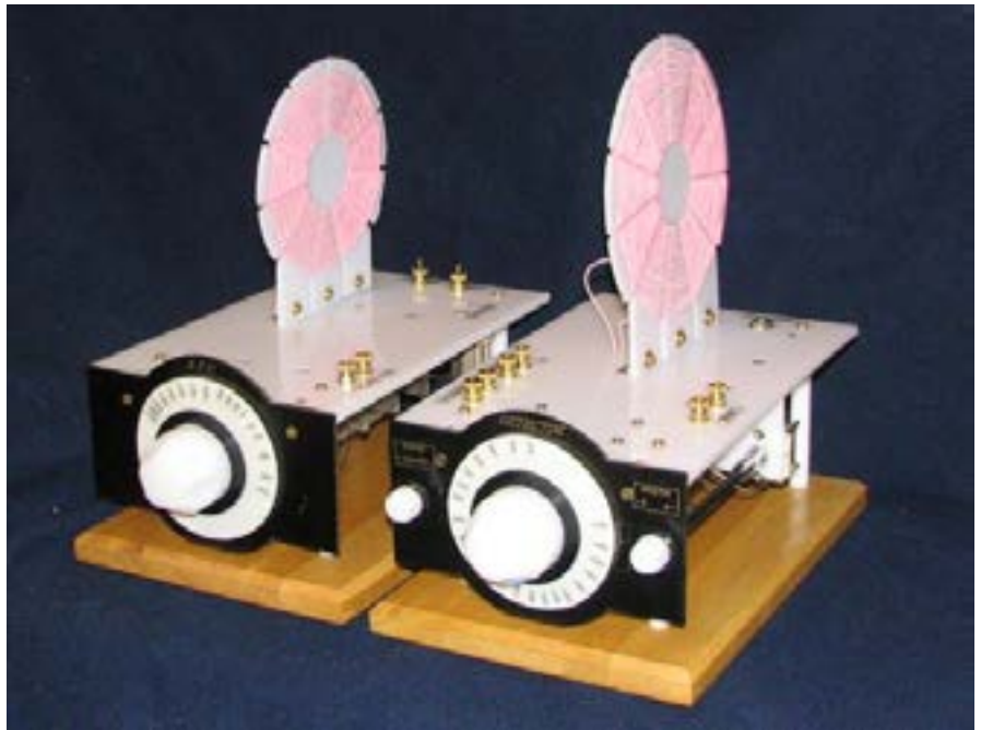
Using modern material and superb craftsmanship, Dave Schmarder N2DS shows how he keeps “old school” radio construction alive. This is his #66 crystal set. Full details on this high-performance set, including schematics and more photographs are found at http://makearadio.com/crystal/66.php . Dave retains the original “breadboard” design on which the components are mounted. This radio is powered by the energy of the radio signal it is receiving. (Courtesy: Makearadio.com)
