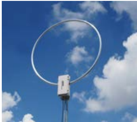
AOR's LA800 amplified loop antenna (left) works from 10 kHz through 500 MHz and measures two feet eight inches across. Control box (right) output is via a BNC jack. A 3.3 foot BNC to BNC patch cable and 33 feet of low loss coax cable is provided. This antenna operates from 12 VDC or via the supplied AC wall adapter.
