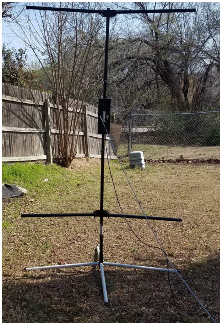
Photo 5 (above) shows the fully assembled antenna using the 20-10-meter center section. (Photo courtesy of the author)
