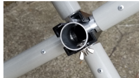
Photo 1 (top left) shows the storage/travel bag for the DX Engineering TransWorld antenna. Photo 2 (bottom left) shows the four fiberglass legs and short mast that comprise the QuadraStand Portable Base. Photo 3 (bottom right) shows the small ring that is held in place by a wing nut and screw. Photo 4 (top right) shows the fully assembled QuadraStand. (Photos courtesy of the author)
