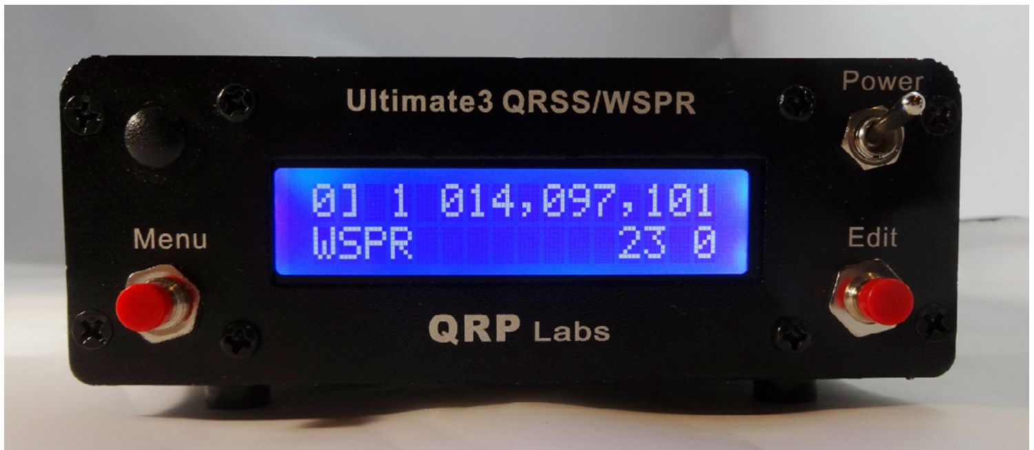
Front panel view of the Ultimate 3S transmitter inside optional case. I elected to leave out the second toggle switch and replaced it with a plastic plug. (Photo: Mark Haverstock)
