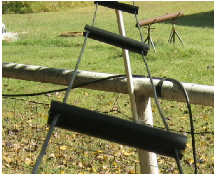
Homemade ladder line, with bare #12 wires. (Photo by author)
