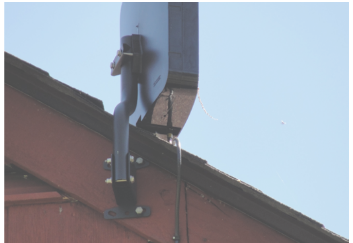
Winegard's FlatWave Air ($100 shipped free from Winegard) VHF/UHF amplified OTA-TV antenna, which comes with its own mount that can be placed on the side of a house, deck or gable end. (KS4ZR photo)
