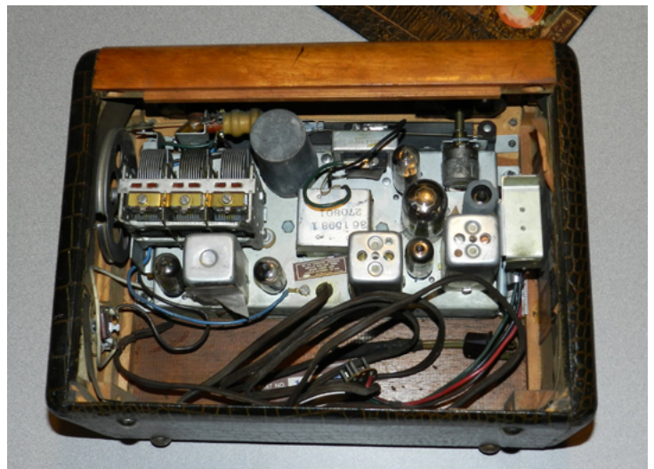
Clean interior as purchased but notice the cracked and taped power cord. (KB8TAD photo)
