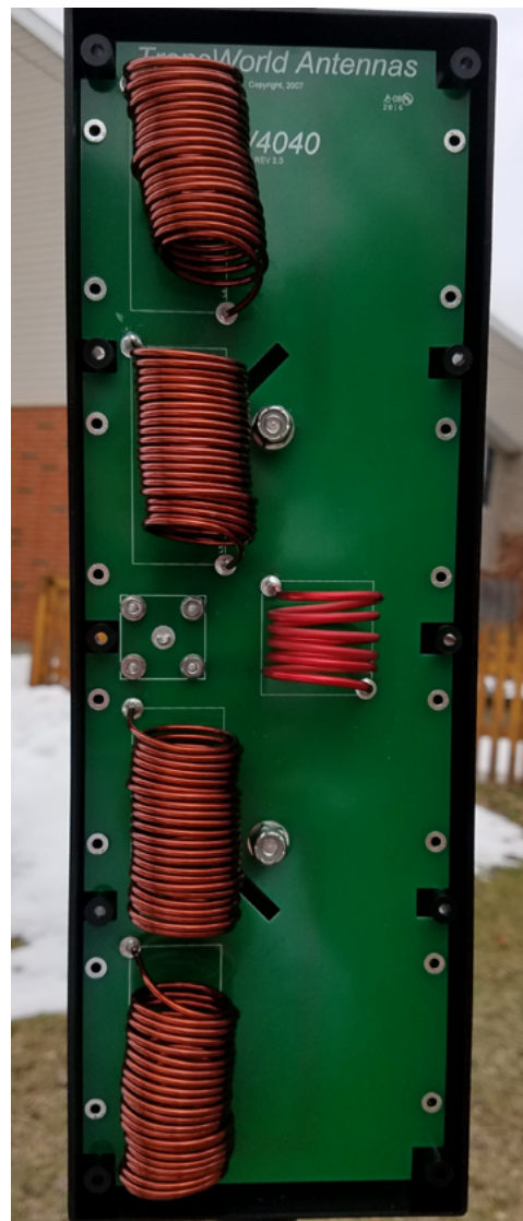
Photo 7 (Left): The antenna in the author's backyard. Photo 8 (Center) Using my MFJ-269C, I determined that the resonant frequency was approximately 7.420 MHz, well outside the 40-meter band. Photo 9 (Right) shows the cover off the antenna's center section with five coils that were adjusted by hand to help tune the antenna. (Photos courtesy of the author)
