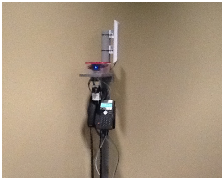
Some proof of concept Go Kits were on display at the Delaware Section Leadership Conference. Support for VOIP telephones, video camera, high-speed data transfers and more are in this affordable and flexible package. (Courtesy of the author)
