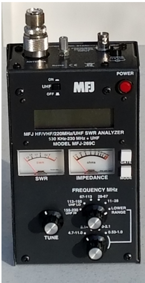
Photo 7 (Left): The antenna in the author's backyard. Photo 8 (Center) Using my MFJ-269C, I determined that the resonant frequency was approximately 7.420 MHz, well outside the 40-meter band. Photo 9 (Right) shows the cover off the antenna's center section with five coils that were adjusted by hand to help tune the antenna. (Photos courtesy of the author)
