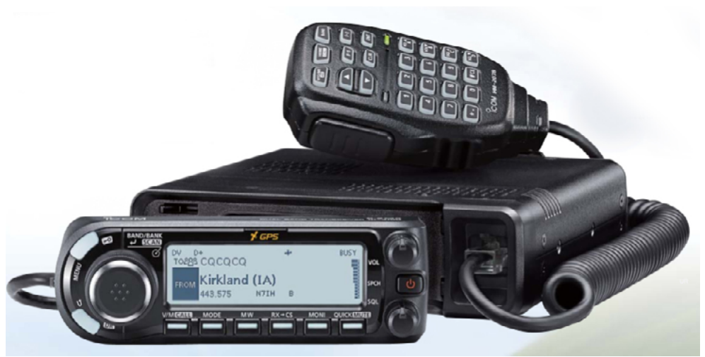
Above: Icom ID-4100a dual-band 2-meter/440 MHz mobile. (Courtesy: Universal Radio)
